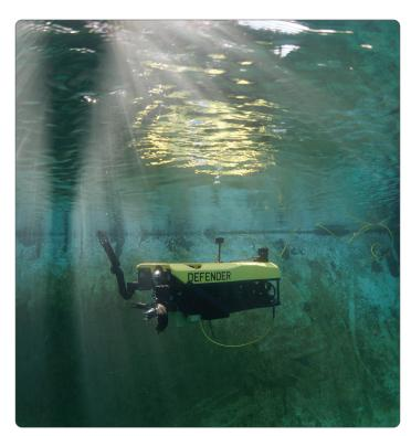
Clearsight's ROV Submersible Inspection Solution helps reduce overall risks associated with underwater diving operations and can reduce overall inspection costs.
