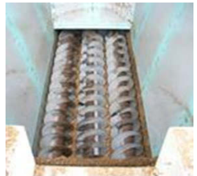
Mounting in discharge screw (wood-fired power plant)
