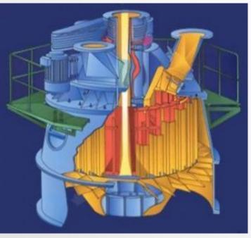
decreases the particle reject rate. Additional features result in a balanced fuel/air ratio pipe-to-pipe.
