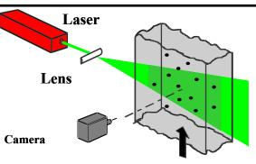
Measurement principal showing laser sheet and CCD rapid imaging.
