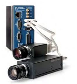
Rapid compact vision system integral to the StackMaster with embedded software for rapidly processing images and derivation of particle size and density.
