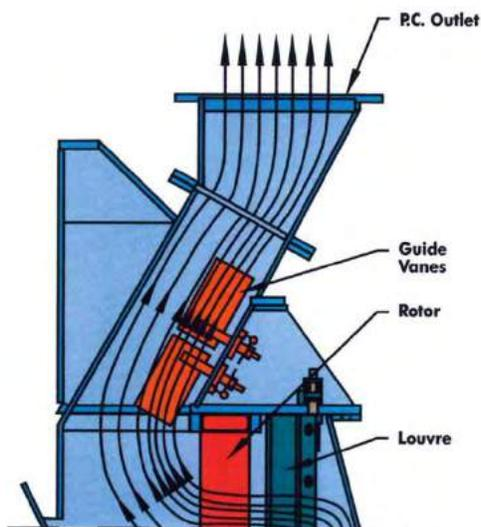
**Figure 19 - HEP coal flow balancing guide vanes**
