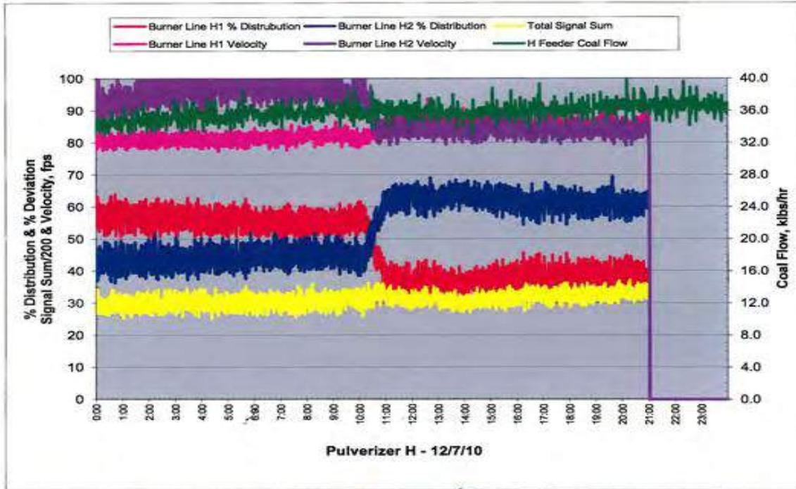
**Figure 8 – Tuning Results Based on a Single Axis Measurement**
