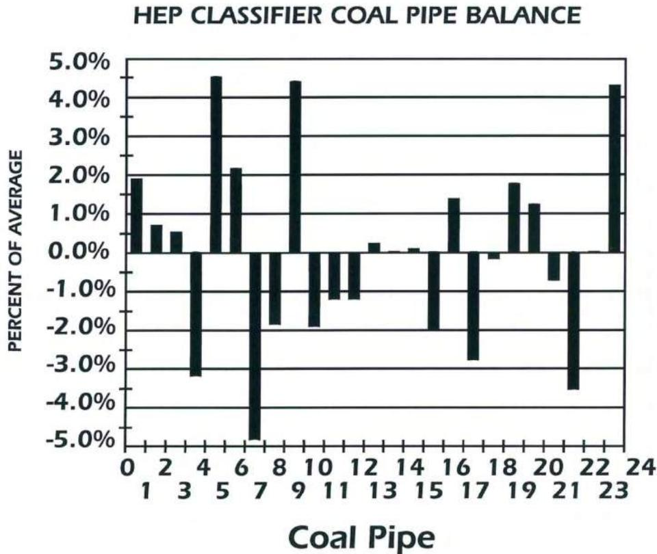
**Figure 20 – Pipe to Pipe Coal flow balance data**
