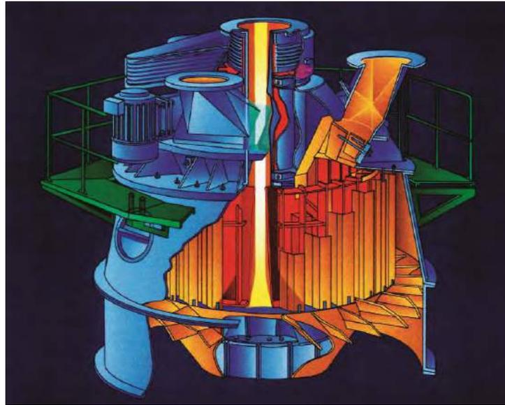
**Figure 18 – General Arrangement of the HEP Dynamic Classifier**
