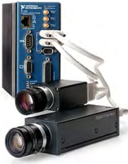
Rapid compact vision system integral to the StackMaster with embedded software for rapidly processing images and derivation of particle size and density.
